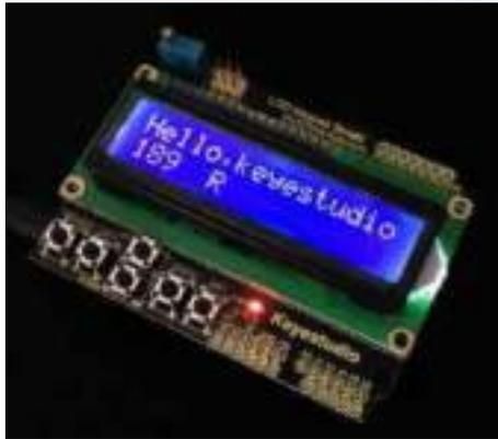
*Fig 11.* LCD Keypad Shield (Rolyi et al, 2019)
