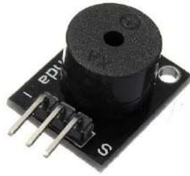
Fig 8. Buzzer-ARDUINO (Mishra & Durgaprasad, 2016)
