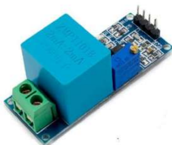
Fig 7. Sensor - ZMPT101B (Meharkure & Kinhekar, 2020)
